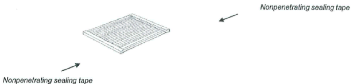
Fig. 8. Sealing of sheet channels under unfavorable operating conditions.
